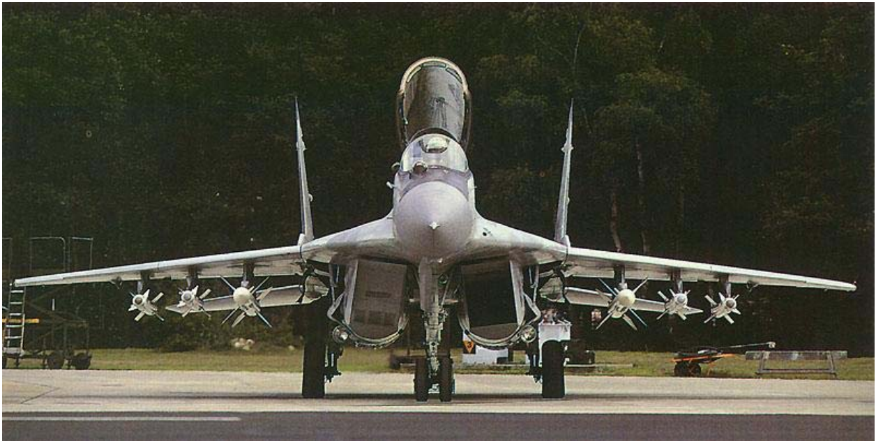
Figure 1: Supersonic Inlet on the MIG-29 (one open & one closed).
